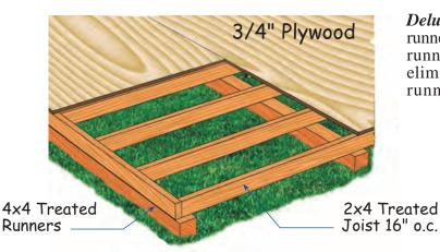
**Deluxe Floor (optional accessory):** 4x4 treated runners can be installed directly on the grass. The runners elevate the floor providing air flow eliminating moisture. 12' wide floor has four runners. Floor covering is 3/4" plywood.
