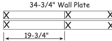
2. Install (3) three 72" wall studs between the 34-3/4" wall plates.
