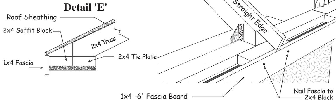
2. Make sure the trusses and gables are plumb and the roof sheathing meets at center of 3rd truss. Starting at the left end of the building, install a 48"x72" OSB roof panel flush with the 1x4 trim on the gable. See detail below. Use 6 common nails spaced 12" apart.
