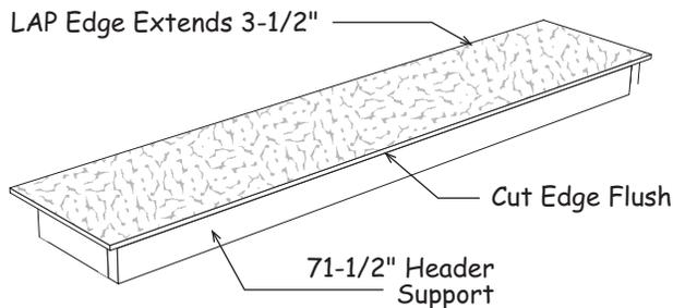
5. Select a 16" wide siding panel with a 'LAP' edge. Install cut edge flush with header support. The 'LAP' edge will extend 3-1/2" beyond the wall frame. Bottom edge will be 3/4" below the bottom plate.
