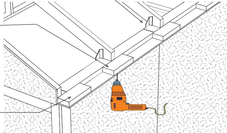
4. Install small primed siding fillers, *packed with the hardware*, over the 2x4 soffit blocks. Siding fillers will be flush with the gable siding. Use 6d galv. nails.
