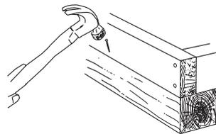
To keep 2x4 frame from moving, toe nail to 4x4.
