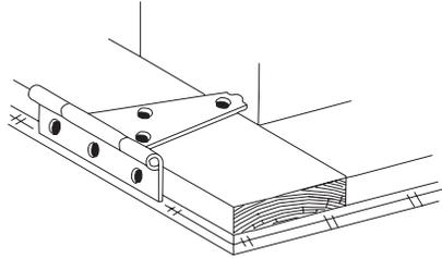
1. Lay the left door with the trim facing up. The siding on the left door extends past the door trim. See detail below.
