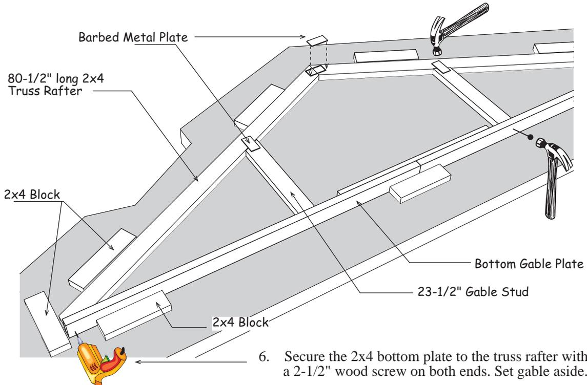
6. Secure the 2x4 bottom plate to the truss rafter with a 2-1/2" wood screw on both ends. Set gable aside.
