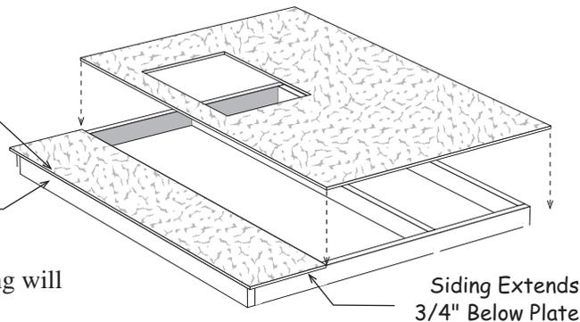
7. Install the last siding panel. The siding will extend 3-1/2" past the wall frame.
