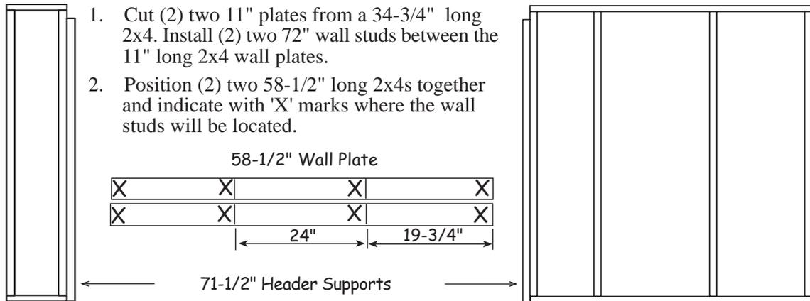
3. Install (4) four 72" wall studs between (2) two 58-1/2" long 2x4 wall plates
