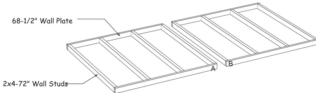
2. Install (8) eight 72" wall studs between the top and bottom plates. Use 10d sinkers, (2) two nails at each stud end. Nail both wall frames together with 10d sinkers.
