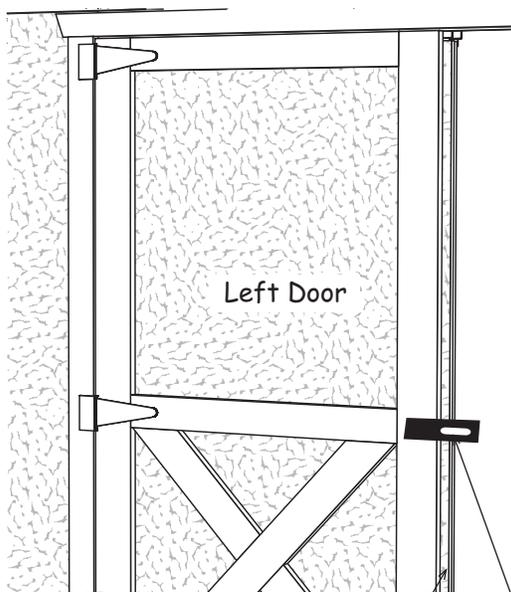
4. Before fastening the hinges to the side trim, temporarily prop the doors in the opening. Leave a space at the top and bottom of the doors and between the doors and the side trim to allow room for the doors to expand due to humidity.
