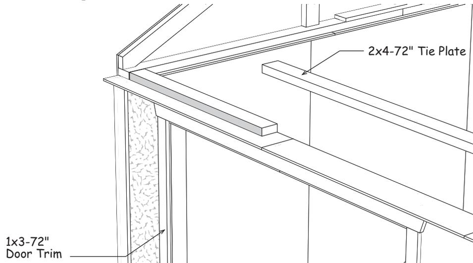
4. Install a 1x3-72" trim board centered across the top door opening and against soffit. The header siding will extend below this trim board. Use 6d galv. nails spaced 12" apart.
