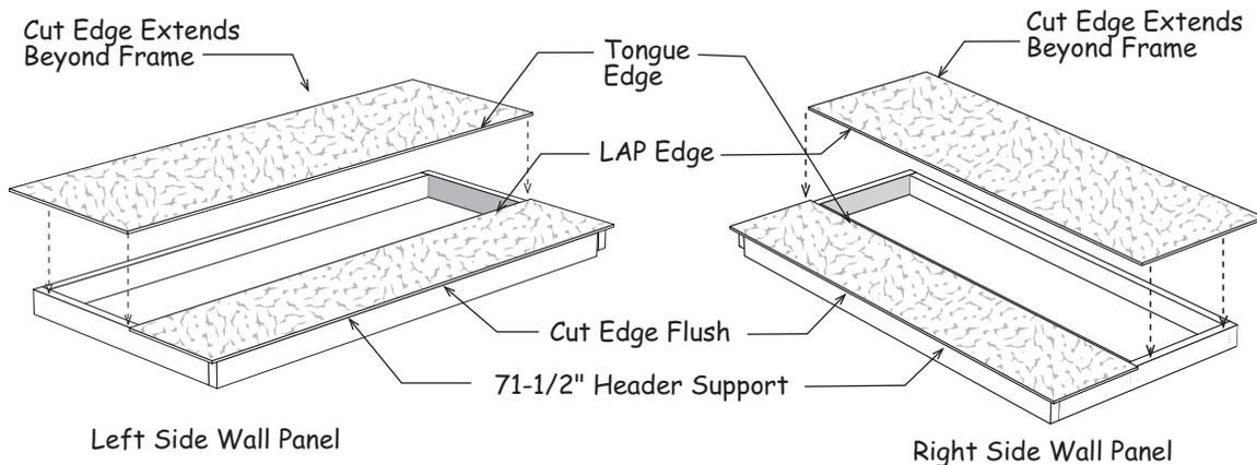
7. Locate a 16" wide siding panel with a 'Tongue' edge and the remaining 24" wide cut panel. Install these on remaining frame. **Make sure header support is oriented to the left.**
