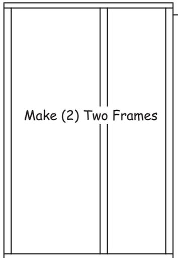
1. Locate (2) two 34-3/4" long 2x4s and position them together. Indicate with 'X' marks where studs will be located..
