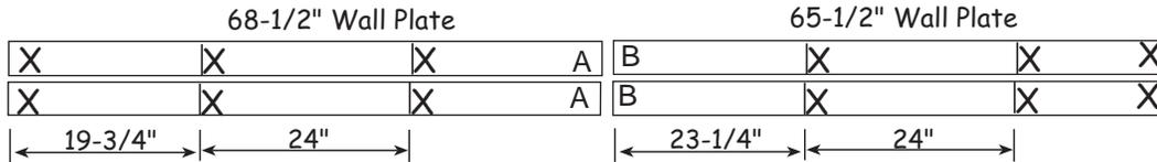
2. Install 72" long wall studs, between the wall plates, over the 'X' marks and where the plates meet. Use (2) two 10d sinkers at each end of stud. Nail wall frames together using 10d sinkers.
