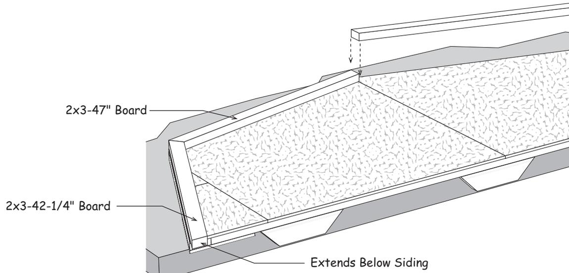
3. Apply 1x4 trim to gable. Install a 47-1/2" long 1x4 at the top of the gable. Install the 1x4 gable trim extending 1/2" above the siding on the gable. When installed later, the roof sheathing will be flush with the top of the trim. Use 6d galv. nails spaced 8" apart.
