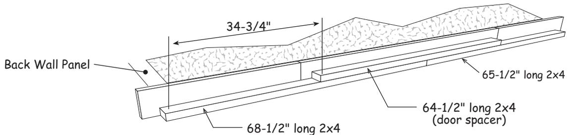
6. Gather (4) four studs and header supports. Install (2) two studs on each end at measurements shown. Install header supports against door spacer. Use 10d sinkers.
