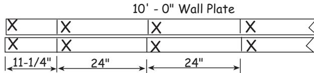
2. Install 72" wall studs between the top and bottom plates.
