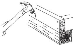
Nail the 2x4s to the 4x4 runners to keep the 2x4 frame from moving.
