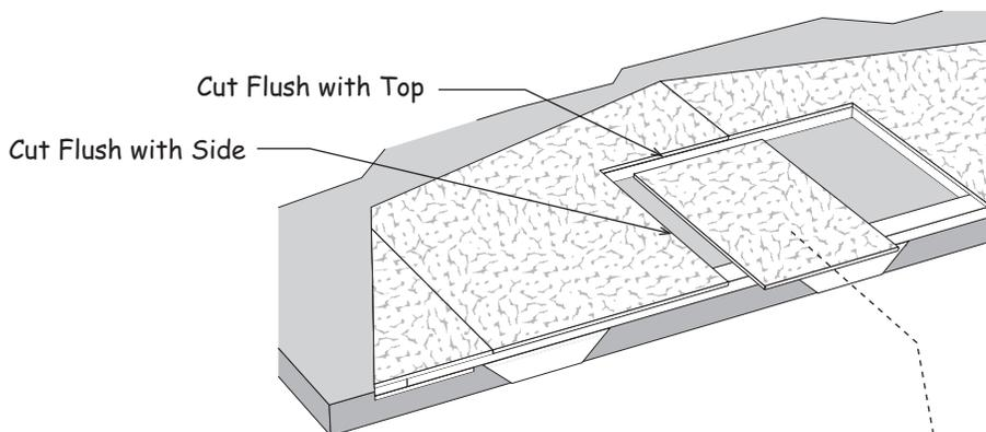
3. Assemble the loft doors. The loft door frames are temporarily held together with corrugated fasteners, this is the back side of the door frame. Place the doors on level surface, face side down. Cut the siding from above step to the size of the door frame. Secure the siding panel to the frame with 1" screws provided.
