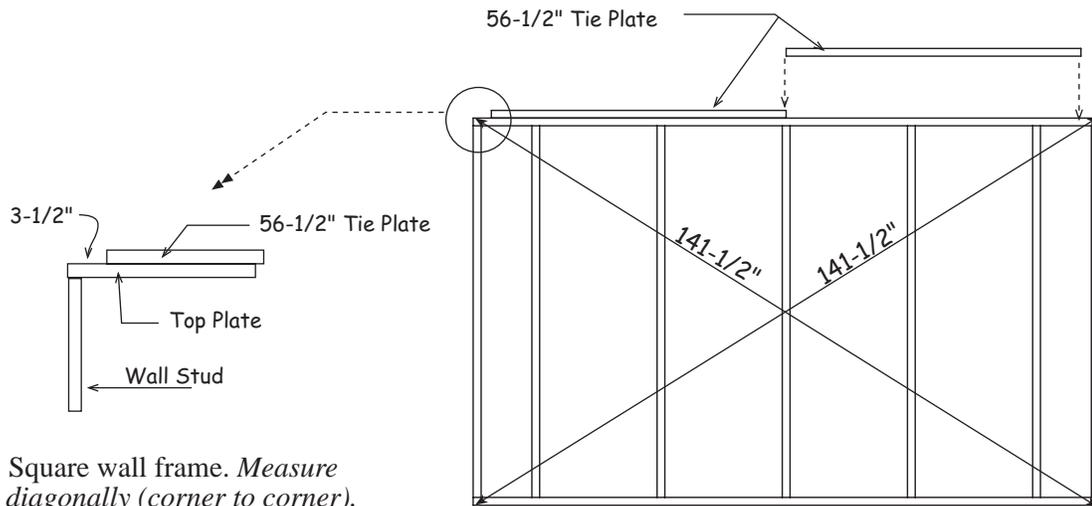
4. Square wall frame. *Measure diagonally (corner to corner).*
