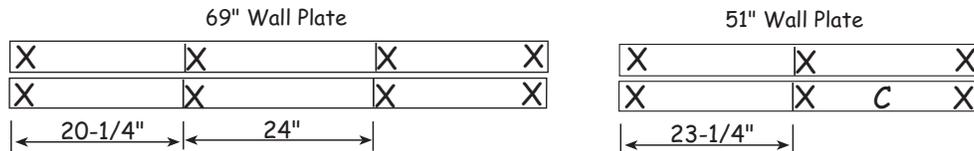
2. Install 72" wall studs between the top and bottom plates. Nail both wall frames together.
