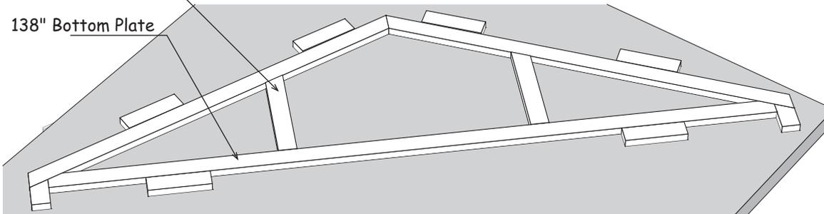
3. Starting from left end install a gable siding with the 'LAP' edge flush with end of gable. The siding should extend 3/4" below the lower 2x4. Nail siding to the frame with 6d galv. nails spaced 8" apart.
