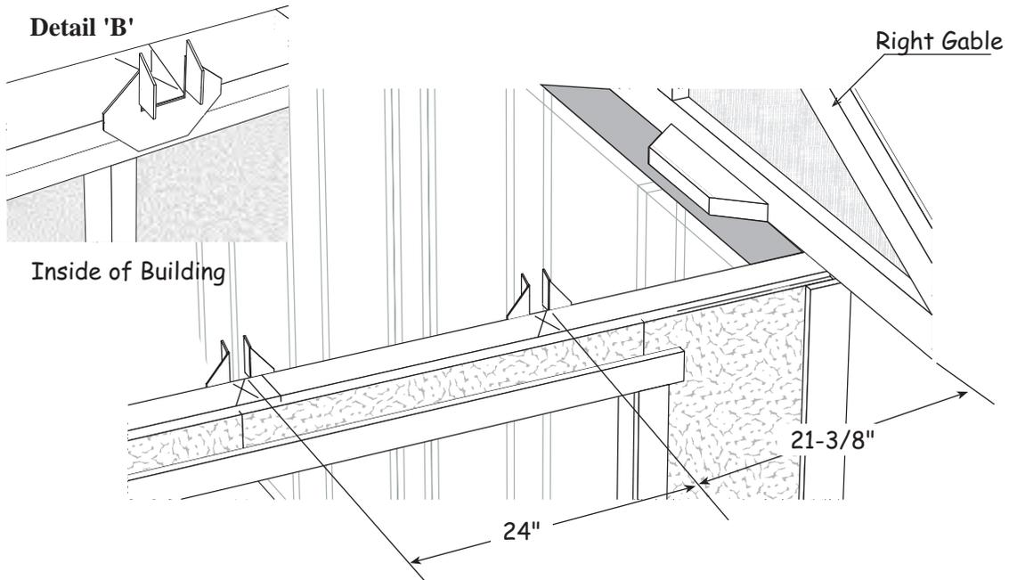
2. Using 1-1/2" hanger nails, install metal hangers to the 2x4 tie plate on the **front wall only**. The opening should line up with the 'X' mark, the bottom of the opening, flush with the 2x4 tie plate. See **Detail 'B'**.
