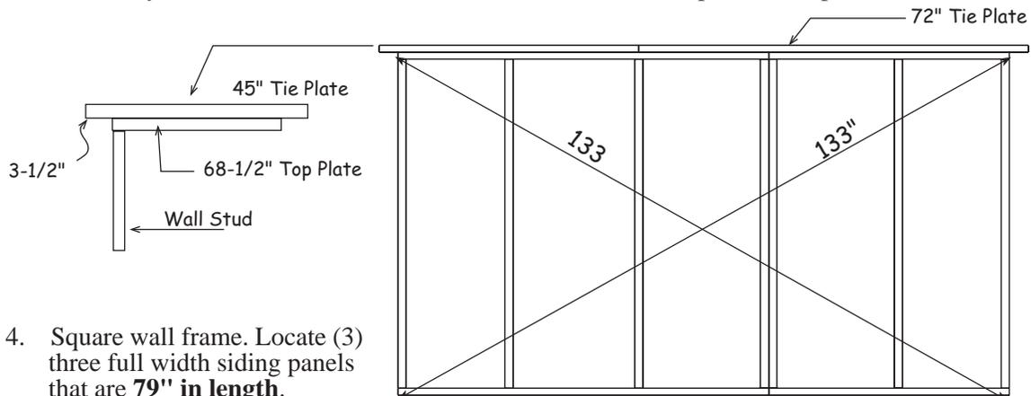
4. Square wall frame. Locate (3) three full width siding panels that are **79" in length**.
