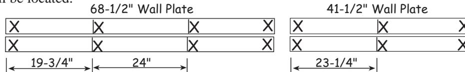
2. Install 72" wall studs between the top and bottom plates. Assemble the frames with 10d sinkers, (2) two nails per stud. Nail both wall frames together with (4) four 10d sinkers (stagger nails on each side of the studs).
