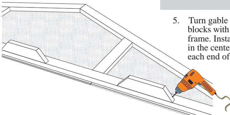
5. Turn gable frame over and install 18" long 2x4 blocks with angle ends to the bottom of the gable frame. Install blocks 21" from each end and one in the center. Use (1) one 2-1/2" long screw on each end of block..
