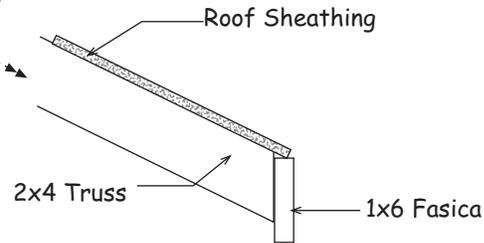
4. Cut to fit a 50" long 1x6 trim board and install flush with the gable trim on the left gable.
