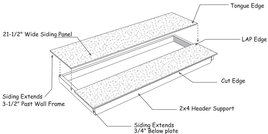
4. Install a pre-cut 16" wide siding panel with the 'cut' edge flush with the 2x4 header support. The siding will extend 3-1/2" beyond the wall frame and 3/4" below the bottom plate.
