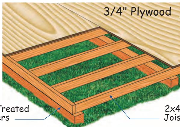
**Deluxe Floor (optional accessory):** 4x4 treated runners can be installed directly on the grass. The runners elevate the floor providing air flow eliminating moisture. 12' wide floor has four runners. Floor covering is 3/4" plywood.
